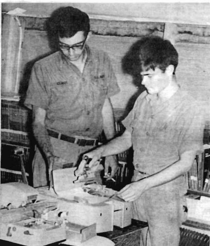
ADDRESSOGRAPH PLATE EMBOSSE AND PRINTER—LTJG R. W. Clark drops the plates into the printer as SN D. C. Lind, PRCP Yeoman, readies to print a Company roster. The printer affords speed in preparing any list, whether original, carbon or stencil.
