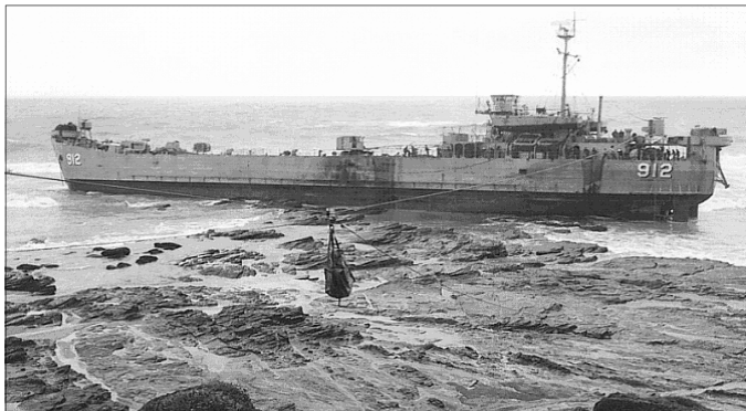
USS Mahnoman County LST-912 ran aground on the rocks just below and to the south of the MCB-8 base camp at about 0117 January 1, 1967. The high-line is connected and a Coaling Bag with Damage Control equipment being sent to the ship.
